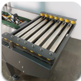
Automatic Box Centering Device with Emergency Stop Switch
