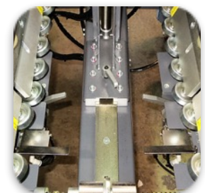
When bottom activation plates are depressed the bottom flap folders are active to close bottom of box.
