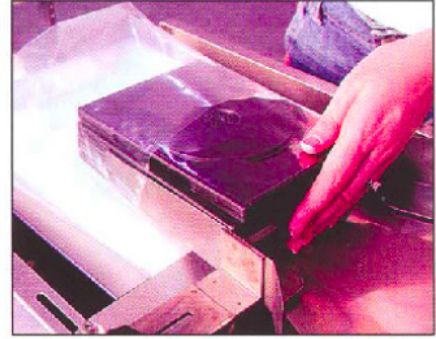
Load product into bag and push forward to tear bag from wicket
